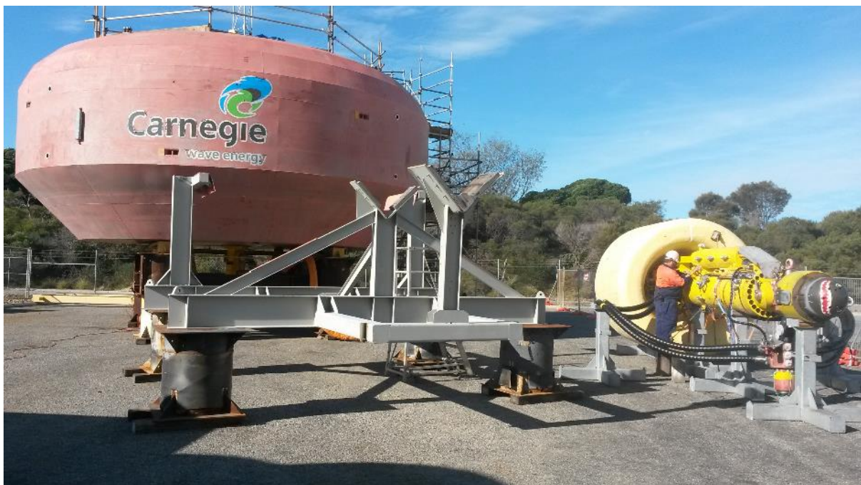
CETO 5 Unit #1 post strip down and inspection works at AMC, Henderson, WA
