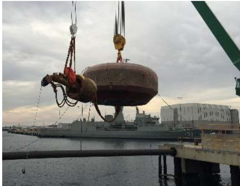
Retrieved CETO Unit being lifted out of the water for planned inspection at the AMC, Henderson, WA
