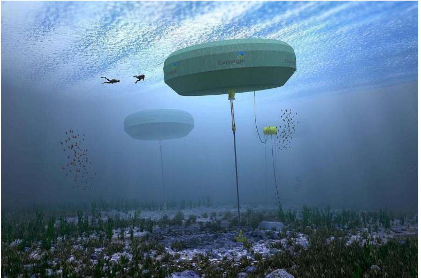
The buoys submerged last year as part of the wave energy system off the coast of Western Australia. The three buoys provided power to a nearby naval base and were the first wave energy system to operate through all four seasons for over 14,000 hours in total. PHOTO: CARNEGIE WAVE ENERGY
